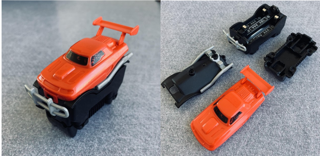
Figure 24. Structural Subsystem assembled (Left), disassembled (Right)
