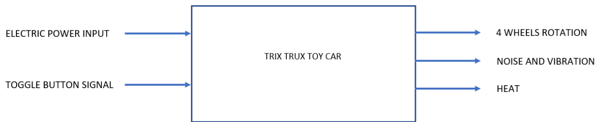
Figure 10. Black Box Diagram of Trix Trux Monster Truck
