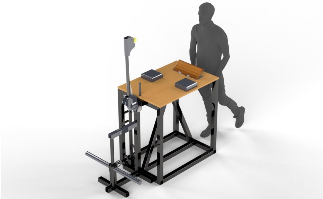
Figure 1. Arm-Wrestle Training Gym Machine (isometric view) next to a 5'8" tall human, for scale.
